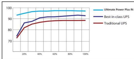
Even at very small loads, where you would expect efficiency to be lower, the UPPRT is still more efficient than other UPS products at full load.
